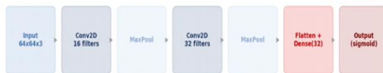
Figure 15.1 — A minimal CNN architecture for blood smear classification (Section 15.6).
